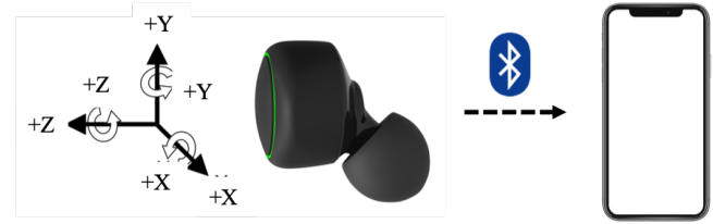
Figure 2: The Nokia Bell Labs eSense headphones [9] (left) connect via Bluetooth and transfer gyroscope and accelerometer data to the smartphone app (right).
