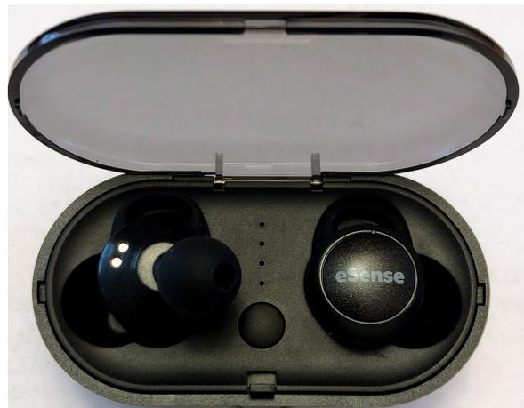
The technique we use to calibrate the IMU is quite simple and more sophisticated methods exist. Essentially we collect 200 accelerometer and gyroscope samples when the earbud is in a known position and then take the average of the values for each axis. This gives the offset that has to be applied to each axis in order to have the appropriate readings: gyro X,Y and Z very close to 0 when the earbud is still and accelerometer X = 0, Y = 0 and Z = -1 when the earbud is facing down.
